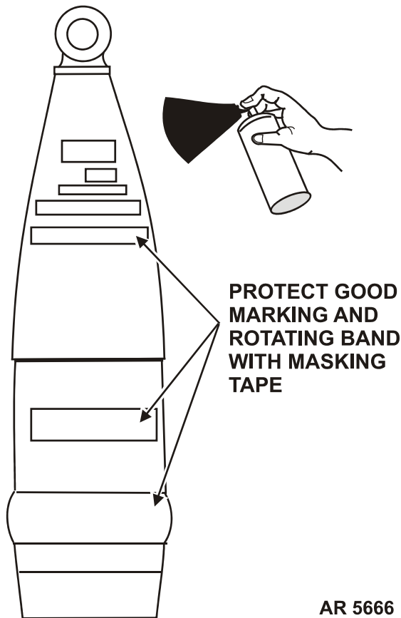
Figure 3-20. Using Spray Paint for Touchup.
